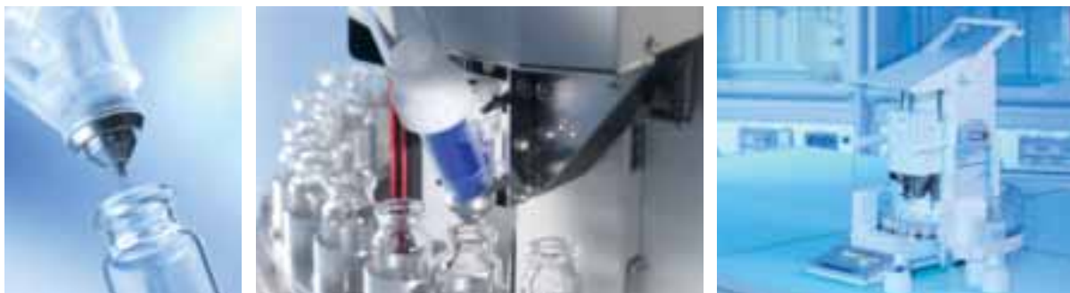
Quantos' dosing head (left) automatically fills vials via a sample handler (middle). The complete instrument (right) includes dosing head, balance and sample handler.
